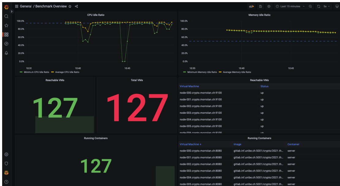
Figure B.1: Grafana dashboard showing the monitoring of the Thetacrypt servers during benchmarking experiments.
