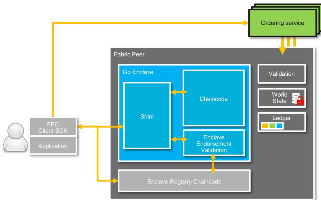
Figure 4.1: FPC Architecture Diagram [2] (Adapted)
